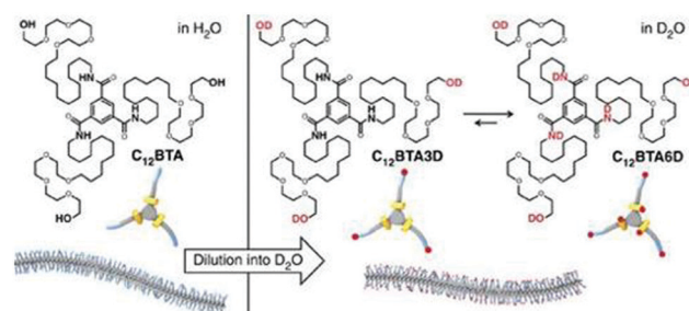
Fig. 14 Schematic representation of the supramolecular polymer formed in water and H/D exchange process in D 2 O. Adapted with permission from ref. 52. Copyright 2017, Nature Publishing Group.
