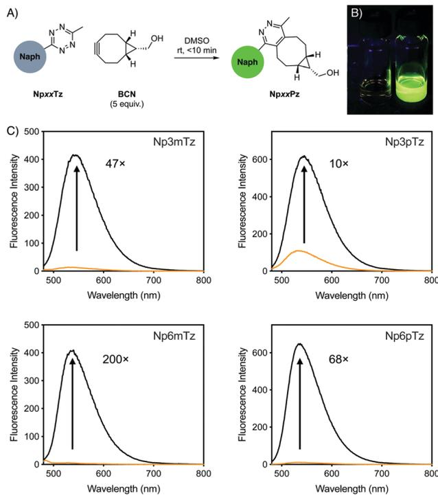
**Fig. 2** (A) Schematic of fluorogenic reaction between naphthalimide (Naph) tetrazines after reaction with BCN to form pyridazine products *in situ*. (B) Photograph of vials of **Np6mTz** (left) and **Np6mPz** (right) in dichloromethane, under 365 nm light. (C) Emission spectra of  $5 \mu\text{M}$  solutions of naphthalimide tetrazines (orange) and the corresponding pyridazine products (black). Numbers indicate the fold turn-on as determined by integration of the spectra.
