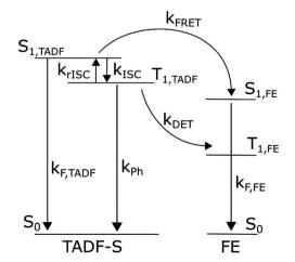
Fig. 1 Energy diagram of a hyperfluorescent system including rates. Nonradiative decay paths are not included, nor energy levels of the host matrix.
