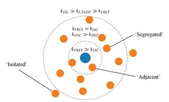
**Fig. 5** A distribution of distances between TADF-S (orange dots) and their nearest neighbour FE (blue dot) leads to different emission lifetimes and mechanisms in optically excited hyperfluorescence systems. Examples of adjacent, segregated, and isolated TADF-S FE pairs are indicated, determined by balances of emission and energy transfer rates at different molecular distances.
