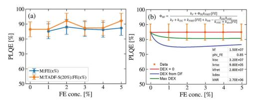
Fig. 4 Photoluminescence quantum efficiencies of hyperfluorescence films at different FE concentrations: (a) experimental data, and (b) fitting to model equation (derivation, choice of fixed rates, and cases for  $k_{dex}$  detailed in the ESI<sup>†</sup>).
