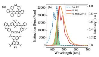
**Fig. 2** (a) Chemical structures of the host matrix DPEPO (M), the TADF sensitiser DDMA-TXO2 (TADF-S) and the fluorescent emitter TBPe (FE), (b) molar extinction spectrum of FE dissolved in toluene (blue), including the normalized photoluminescence spectra of TADF-S (orange) and FE (red). The overlap between TADF-S emission and FE extinction is highlighted in green resulting in a Förster radius  $R_{\rm FRET}$  of 3.0 nm.
