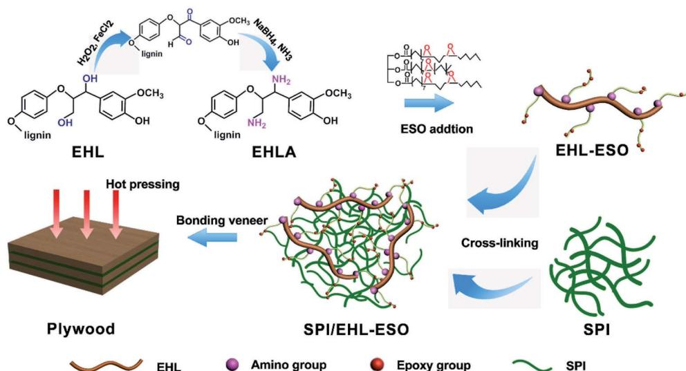
Scheme 1 The crosslinking reactions process of SPI/EHL-ESO adhesives.
