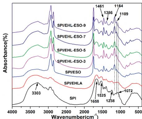
Fig. 5 FTIR curves of different soy protein-based adhesives.
