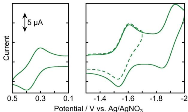
Fig. 4 Cyclic voltammograms of Os (0.5 mM) in an Ar-saturated DMA solution containing Et<sub>4</sub>NBF<sub>4</sub> (0.1 M) as a supporting electrolyte with a Ag/AgNO<sub>3</sub> (10 mM) reference electrode. Scan rate was 0.2 V s<sup>-1</sup>.
