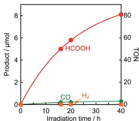
Fig. 8 Photocatalytic formation of HCOOH (●), CO (◆), and H<sub>2</sub> (■): CO<sub>2</sub>-saturated DMA solutions (2 mL) containing Os (50 μM), Ru(CO) (50 μM), and BI(OH)H (0.2 M) were irradiated with 725 nm light.
