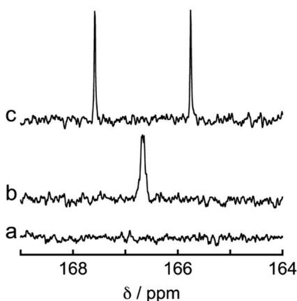
Fig. 9 <sup>13</sup>C{<sup>1</sup>H} NMR spectra of a DMF-*d*<sub>7</sub> solution of **Os** (0.5 mM), **Ru(CO)** (50  $\mu\text{M}$ ), and BI(OH)H (0.2 M) under a <sup>13</sup>CO<sub>2</sub> (447 mmHg) atmosphere (a) before and (b) after 60 h of irradiation. (c) <sup>13</sup>C NMR spectrum without <sup>1</sup>H decoupling of the same solution after irradiation.
