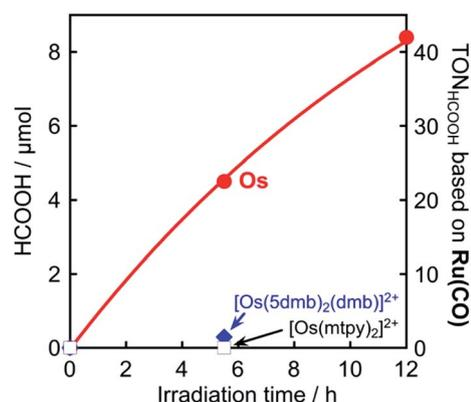
Fig. 11 Photocatalytic formation of HCOOH using light at  $\lambda_{\text{ex}} > 770$  nm and **Os** (●), [Os(5dmb)<sub>2</sub>(dmb)]<sup>2+</sup> (◆), or [Os(mtpy)<sub>2</sub>]<sup>2+</sup> (□) as a redox photosensitizer: CO<sub>2</sub>-saturated DMA solutions (4 mL) containing osmium(II) photosensitizer (0.6 mM), **Ru(CO)** (50  $\mu\text{M}$ ), and BI(OH)H (0.2 M) were irradiated.
