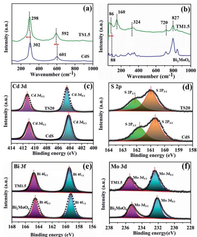
Fig. 2 (a) Raman spectra of TS1.5 and CdS; (b) Raman spectra of TM1.5 and  $\text{Bi}_2\text{MoO}_6$ ; high-resolution XPS spectra of the core levels of Cd 3d (c), S 2p (d) over the CdS and TS20 samples and Bi 3f (e) and Mo 3d (f) over the  $\text{Bi}_2\text{MoO}_6$  and TM1.5 samples.
