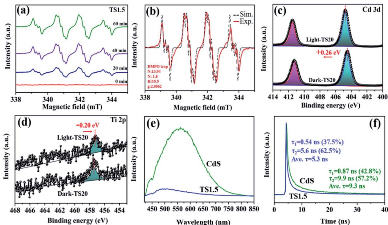
Fig. 5 (a) *In situ* ESR spectra of TS1.5 monitored during the photocatalytic reaction with the increase of reaction time; (b) simulation results of the amine free-radical; XPS spectra of Cd 3d (c) and Ti 2p (d) in the TS1.5 sample under dark conditions and irradiation at 402 nm; PL emission (e) and time-resolved photoluminescence spectra (f) of TS1.5 and CdS samples.
