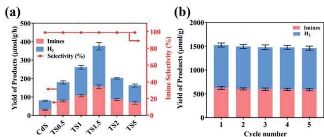
Fig. 3 (a) Photocatalytic activity of different samples for benzylamine oxidation and  $\text{H}_2$  generation under visible light irradiation ( $\lambda \geq 420$  nm); (b) recycling tests over the TS1.5 composite for photocatalytic benzylamine oxidation integrated with  $\text{H}_2$  production (each cycle is 4 h).
