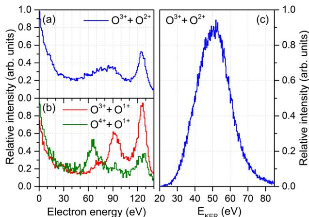
Fig. 1 Electron energy spectra of  $O_2$  irradiated with intense XFEL pulses ( $h\nu = 665$  eV) recorded in coincidence with the  $O^{3+} + O^{2+}$  final state (panel a), the  $O^{3+} + O^{1+}$  and the  $O^{4+} + O^{1+}$  final states (panel b), together with the ion kinetic energy release spectrum for the  $O^{3+} + O^{2+}$  case (panel c). The relative strength of the three breakup channels is  $O^{3+} + O^{2+}$ : 1,  $O^{3+} + O^{1+}$ : 0.66, and  $O^{4+} + O^{1+}$ : 0.14.
