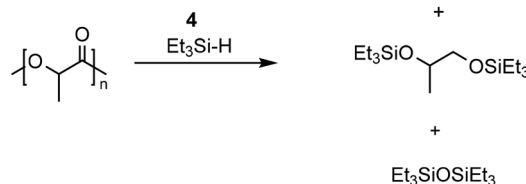
Scheme 3 Reduction of PLA into silylated alcohols with Et 3 SiH and 4 .
