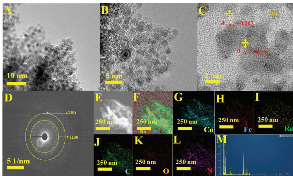
**Fig. 3** (A and B) Different magnification TEM images. (C) High-resolution TEM image with lattice fringe. (D) SAED patterns. (E) STEM image. (F) The corresponding TEM elemental maps of (G) Co, (H) Fe, (I) Ru, (J) C, (K) O and (L) N elements. (M) TEM EDX spectrum of Ru MOF FeCo nanoarrays.
