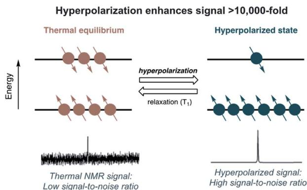
Fig. 1 Hyperpolarization of the nuclear-spin population to enhance NMR signals.
