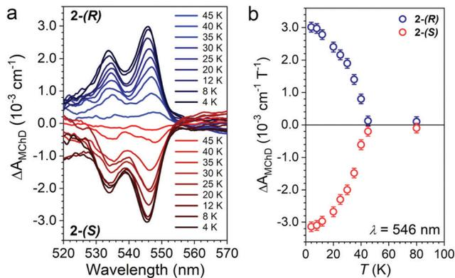
Fig. 6  $\Delta A_{\text{MChD}}$  at different temperatures (see legend) for both **2-(R)** and **2-(S)** in the 520–570 nm range (a). Temperature dependence of  $\Delta A_{\text{MChD}}$  at  $\lambda = 546$  nm for both enantiomers (b).
