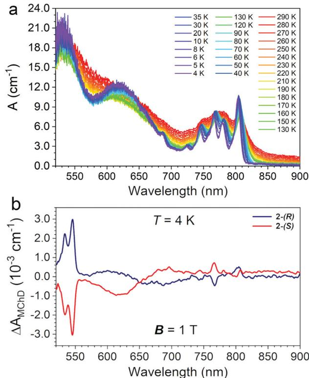
Fig. 5 Temperature variation (see legend) of the absorption coefficient  $A$  (cm<sup>-1</sup>) for an oriented single crystal of **2-(R)** (a).  $\Delta A$  at 4.0 K recorded on single crystals of **2-(R)** and **2-(S)** (see legend) oriented in the same direction (b).
