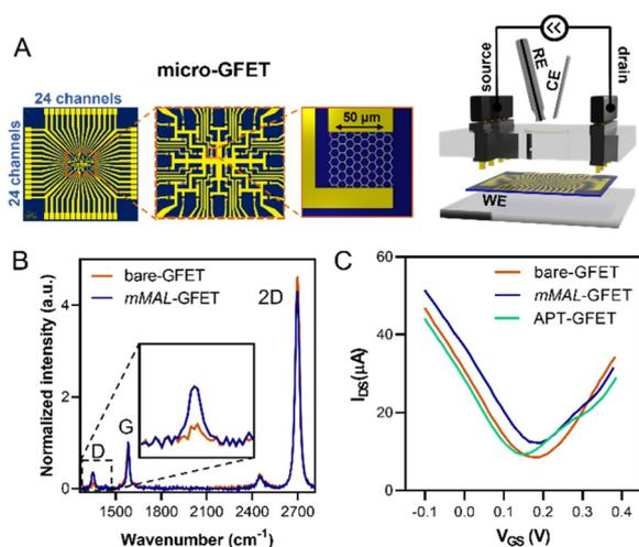
**Fig. 5** Micro-GFET electrochemical functionalisation characterisation. (A) Schematic of the micro-GFET device and electrochemical setup. (B) Raman spectra of the pristine bare-GFET and mMAL-GFET. (C) Transfer curves recorded on the micro-GFET recorded after each step of functionalisation.
