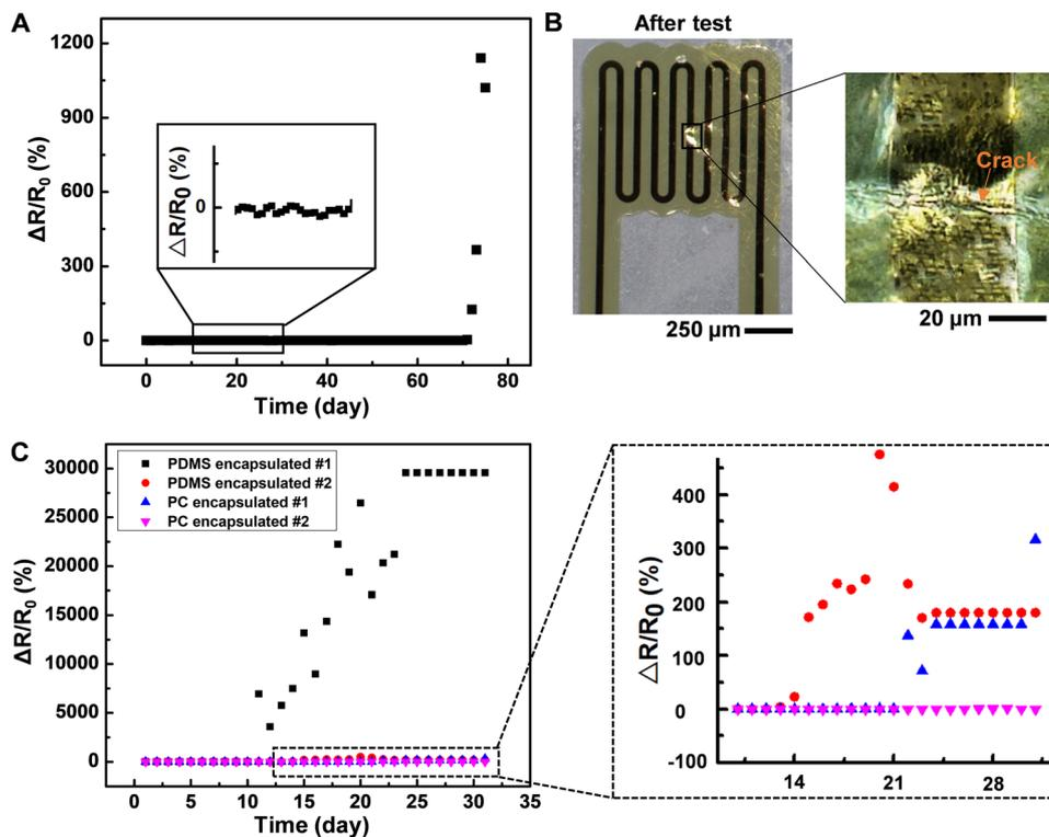
Fig. 4 Encapsulation capability of the soft pressure sensor. (A) Fractional resistance change of the rectangular pressure sensor tested under a hydrostatic pressure of 10 MPa in the pressure vessel filled with DI water. (B) Optical microscope images of the rectangular sensor after the test. (C) Comparison between the encapsulation capabilities of the PDMS film and Parylene C film for pressure sensors under 35 PSU salinity level and 10 MPa hydrostatic pressure conditions in the pressure vessel.
