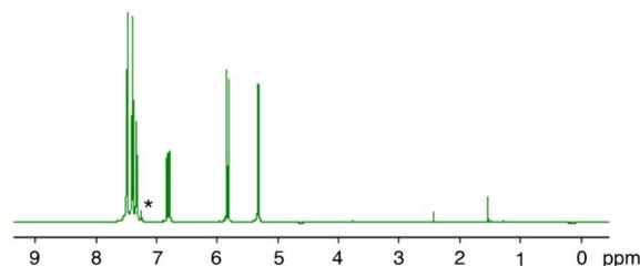
Fig. 2  $^1\text{H}$  NMR spectrum of the styrene recovered by the pyrolysis of the waste PS foam. Solvent:  $\text{CDCl}_3$ . \*  $\text{CHCl}_3$ .
