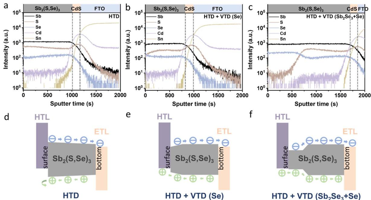
Fig. 4 Depth profiling via TOF-SIMS of the  $\text{Sb}_2(\text{S,Se})_3$  films and energy band structures of the corresponding solar devices: (a and d) HTD, (b and e) HTD + VTD (Se), and (c and f) HTD + VTD ( $\text{Sb}_2\text{Se}_3 + \text{Se}$ ).
