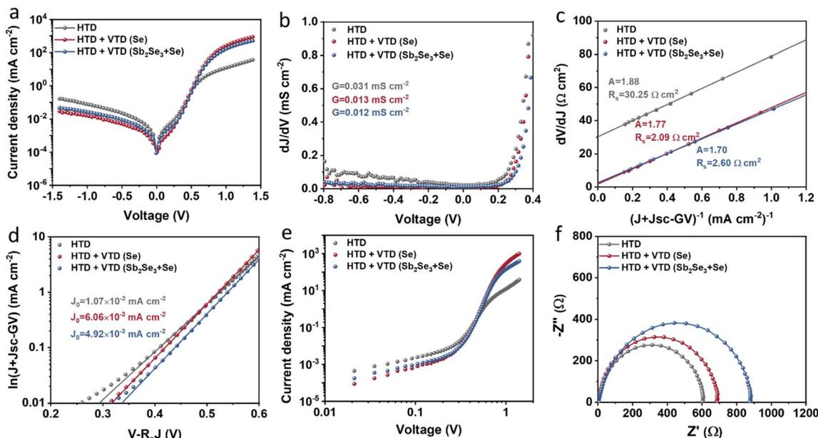
Fig. 5 Charge transport behaviors of the representative  $\text{Sb}_2(\text{S,Se})_3$  devices: (a) semi-logarithmic dark  $J$ - $V$  plots, (b)  $dJ/dV$  versus  $V$  plots for  $G$ , (c)  $dV/dJ$  versus  $(J + J_{sc} - GV)^{-1}$  plots for extracting  $R_s$  and  $A$ , (d)  $\ln(J + J_{sc} - GV)$  versus  $V - R_s J$  plots for extracting  $J_0$ , (e) SCLC spectra derived from the dark  $J$ - $V$  curves, and (f) Nyquist plots extracted from IS.
