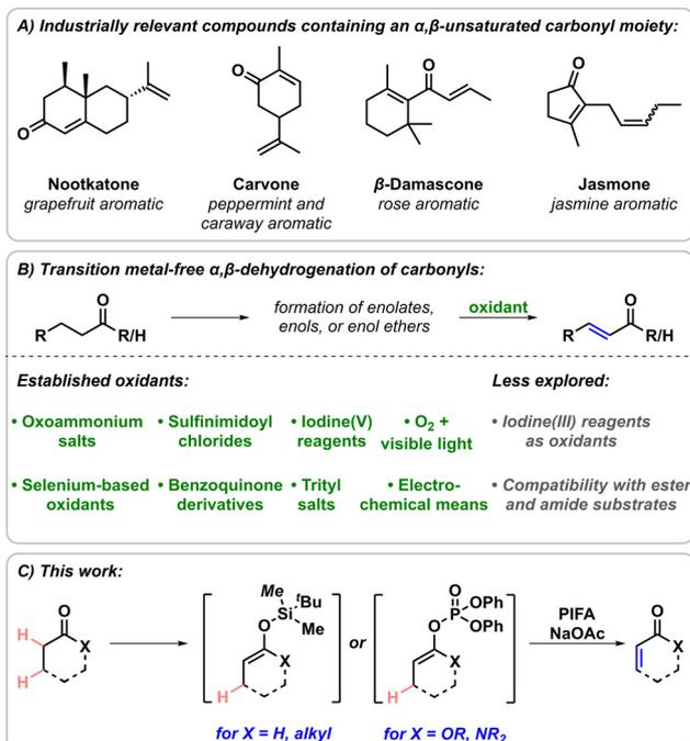
**Scheme 1** (A) Relevance of  $\alpha,\beta$ -unsaturated carbonyl compounds. (B) Previous examples of transition metal-free carbonyl dehydrogenation. (C) This work.
