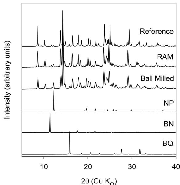
Fig. 6 XRPD data of rBN/BQ/NP at a 2:1:2 mole ratio subjected to BM and RAM shown in comparison to the reference powder data calculated from the published single crystal structure of rBN/BQ/NP and experimental powder data of NP, rBN, and BQ. BM was performed at 30 Hz for 30 minutes. RAM was performed at 90g for 90 minutes. 470 mg of total solids were used for the BM experiments while 490 mg of total solids were used for the RAM experiments.
