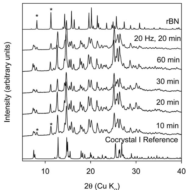
Fig. 2 XRPD data of rBN/BQ ball milled at a 1:1 mole ratio shown in comparison to the reference powder data calculated from the published crystal structure of cocystal I and the experimental powder data of rBN. Ball milling was done for different times at 25 Hz except for the one sample indicated in the figure. 480–490 mg of total solids were used for the experiments. The peaks marked with “\*” at 8° and 11.1° 2θ are associated with unreacted rBN.
