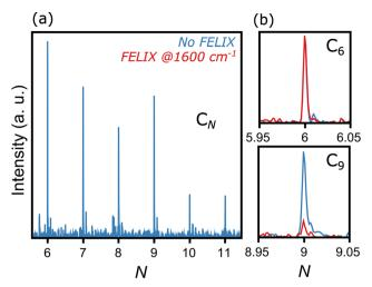
Fig. 2 Representative mass spectrum of  $C_N$  clusters ionized by 118 nm laser light, produced by the desorption and fragmentation of C<sub>60</sub> molecules. Left panel: No FELIX excitation. Right panel: Comparison of intensities without (blue) and with (red) FELIX irradiation at 1600  $\mbox{cm}^{-1}$  for  $\mbox{C}_{6}$ (top) and C9 (bottom).
