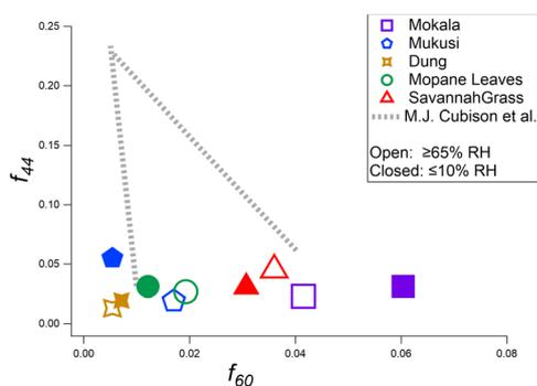
Fig. 3 Primary BBOA composition displayed via  $f_{60}$  versus  $f_{44}$  from ACSM OA mass spectra of primary BBOA mass under dry ( $<10\%$  RH, closed symbols) or elevated humidity ( $\geq 65\%$  RH, open symbols) conditions in the dark for all fuels used in this work.
