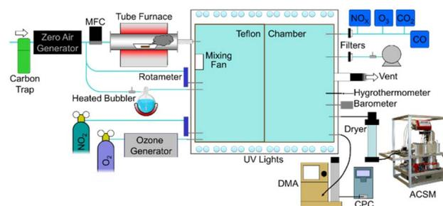
Fig. 1 Experimental laboratory schematic adopted from Pokhrel *et al.*<sup>60</sup> Particle aging was studied in a 9.0 m<sup>3</sup> smog chamber at the North Carolina Agricultural and Technical State University (NC A&T University). The setup features a tube furnace that allows temperature control, where  $\sim 0.050$ – $0.500$  gram fuel samples were combusted at 450 °C. The chamber has been fully characterized in a prior study.<sup>66</sup>
