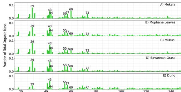
**Fig. 2** Representative average OA mass spectra from the ACSM of controlled combustion experiments conducted without the introduction of humidity (RH < 10%) or external oxidants. Note data represents primary aerosol emissions from burning (A) mokala, (B) mopane leaves, (C) mukusi, (D) savannah grass, and (E) dung. ACSM measurements were taken within the first hour after combustion and is representative of data averaged over 15–20 min, which is 1 data point.
