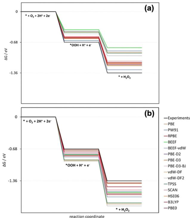
Fig. 10 Free-energy diagrams at 0 V vs. RHE for hydrogen peroxide production on the ideal catalyst using several xc-functionals. (a) Gas-phase corrections are not included. (b) Only the errors in  $O_2$  are corrected. In black in both panels is the experimentally expected profile, obtained when both errors are corrected. Reproduced from ref. 27, licensed under CC BY 4.0 (<https://creativecommons.org/licenses/by/4.0/>).
