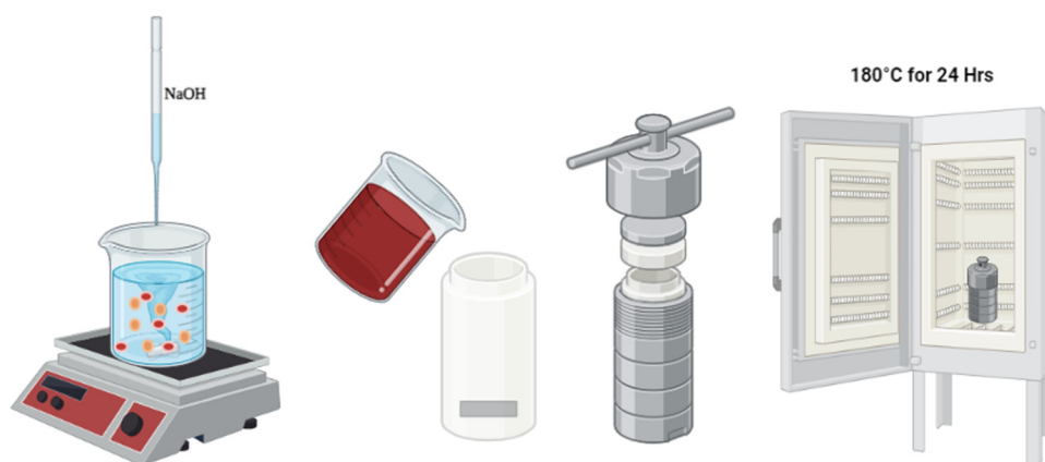
Scheme 1 Hydrothermal synthesis of the \text{CoFe}_2\text{O}_4/\text{Ni} foam electrodes.
