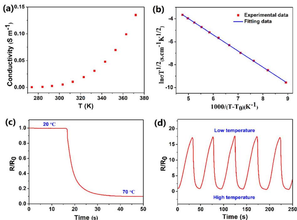
**Fig. 4** (a) Temperature dependence of the conductivity of the PIL (from 273 K to 373 K). (b) VTF fitting curve of the conductivity of the PIL. (c) Time-dependent resistance evolution of the PIL for detecting temperature changes. (d) Time-dependent resistance evolution of the PIL for detecting regular temperature changes.
