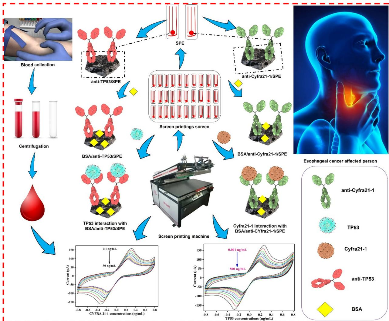
**Scheme 1** The fabrication of SPE and the development of two immunoplatfroms, *i.e.*, BSA/anti-CYFRA21-1/SPE and BSA/anti-TP53/SPE for the dual detection of CYFRA21-1 and TP53 cancer biomarkers, respectively, in the serum samples of esophageal-affected cancer patients.
