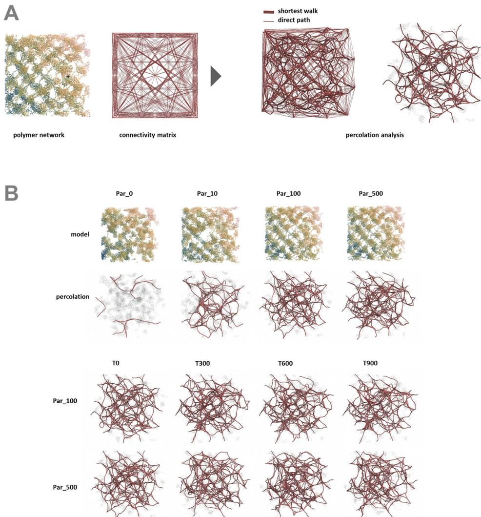
Fig. 4 Percolation was assessed within each polymer network at multiple time steps under deformation. (A) Percolation was measured by comparing the number of possible paths between distant points on the network's periphery to the number of viable shortest walks through the network between those points. (B) Each network demonstrated different degrees of connectivity, and the number and form of viable paths through the network changed under deformation.
