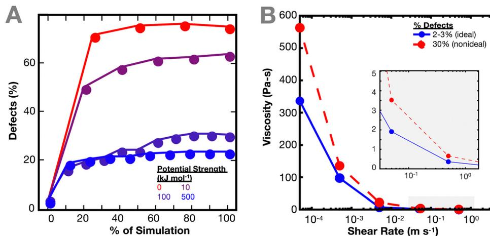
Fig. 3 Effect of defects on viscosity of polymer network. (A) Defects in network based on individual crosslinks for  $10^{-9}$  fs<sup>-1</sup> engineering strain rate across different interaction potentials. The defects increase over simulation time. (B) Comparison of viscosity of network with 2–3% initial defects versus ~30% initial defects for an interaction potential of 100 kJ mol<sup>-1</sup>.
