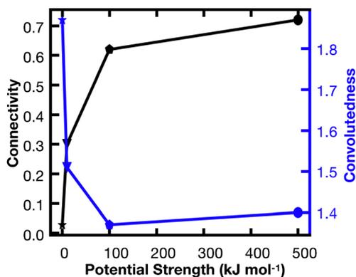
Fig. 5 Connectivity vs. convolutedness for models with interaction potentials of 0, 10, 100, 500 kJ mol<sup>-1</sup>. As the interaction potential increases, the connectivity of the network goes up, while the convolutedness goes down. This implies that a stronger potential holds the network together more robustly.
