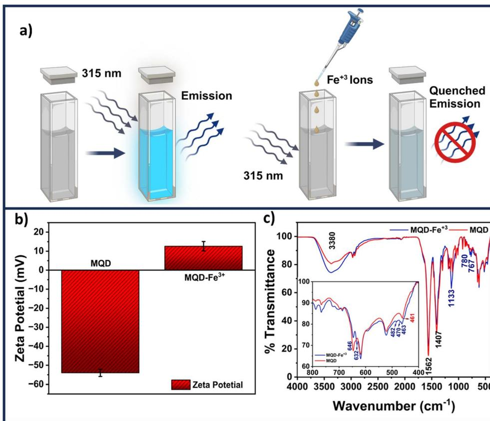
Fig. 7 (a) Schematic representing the mechanism of fluorescence quenching of MQDs in the presence of Fe<sup>3+</sup> ions, (b) zeta potential measurements of MQDs and MQD with Fe<sup>3+</sup> ions in ultrapure water, (c) FTIR spectrum of MQDs and MQD with Fe<sup>3+</sup> ions.
