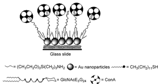
Fig. 25 Diagrammatic representation of the self-assembled multilayer system used for studying biomolecular binding. Reproduced from ref. 72 with permission from [ACS Publications], copyright [1995].
