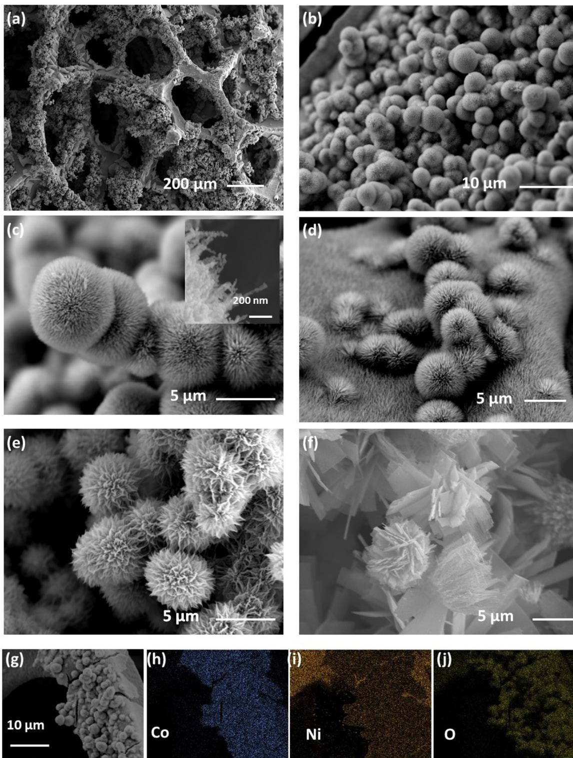
**Fig. 1** SEM images of different Ni–Co oxide structures anchored on Ni foam, (a–d) low and high magnifications of the NCO 120 structure, (e) NCO 150, (f) NCO 180, and (g–j) EDX analysis of the NCO 120 structure.
