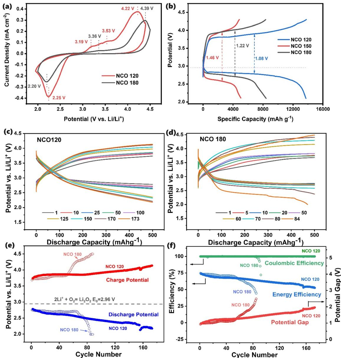
**Fig. 4** (a) CV analysis @0.2 mV s<sup>-1</sup> and (b) full discharge–charge @100 mA g<sup>-1</sup>, and selected discharge–charge curves of (c) NCO 120 and (d) NCO 180 cathode-based LABs operated at 100 mA g<sup>-1</sup> for a limited capacity of 500 mA h g<sup>-1</sup>. (e and f) Cycle life and performance analysis of LABs with NCO 120 and NCO 180 based cathodes with cut-off discharge capacity of 500 mA h g<sup>-1</sup> with 1 M LiTFSI dissolved in TEGDME electrolyte.
