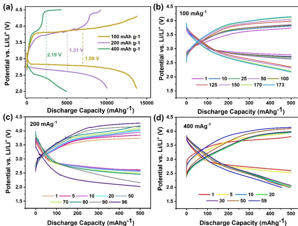
Fig. 5 Electrochemical performance analysis of NCO 120 cathode-based LABs under different current densities: (a) full discharge–charge capacity, selected discharge–charge curves under a current density of (b)  $100 \text{ mA g}^{-1}$ , (c)  $200 \text{ mA g}^{-1}$ , and (d)  $400 \text{ mA g}^{-1}$ .
