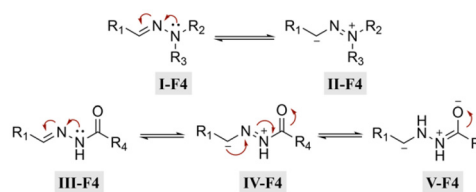
Fig. 4 Scheme showing the electron delocalization in alkyl and acyl hydrazones.
