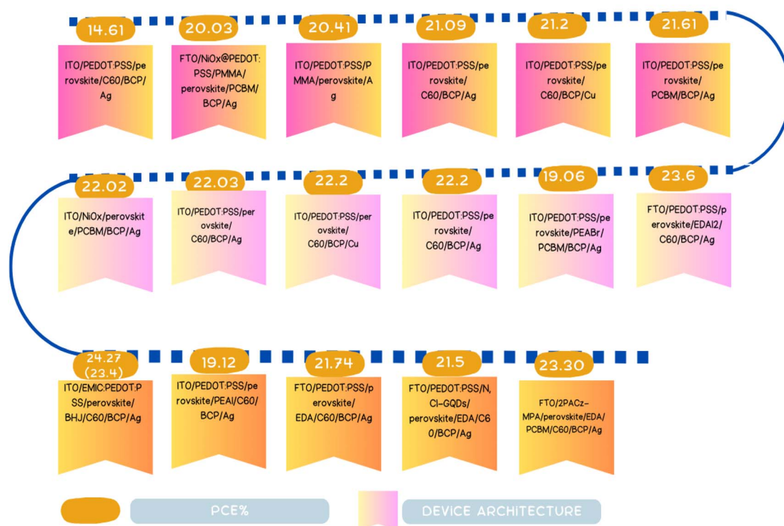
Fig. 11 Recent device performance of tin–lead mixed PSCs.
