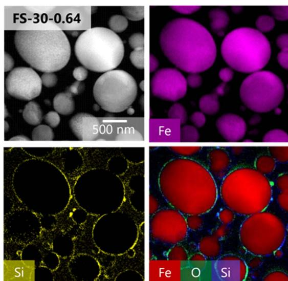
Fig. 6 TEM image and elemental mapping of the cross-section of Fe@SiO<sub>2</sub> particles (FS-30-0.64).
