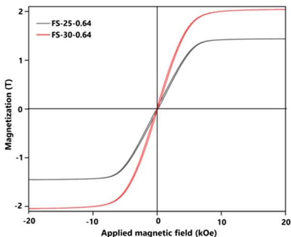
Fig. 9 Magnetic hysteresis loop values of prepared Fe@SiO<sub>2</sub> particles from samples FS-25-0.64 and FS-30-0.64.
