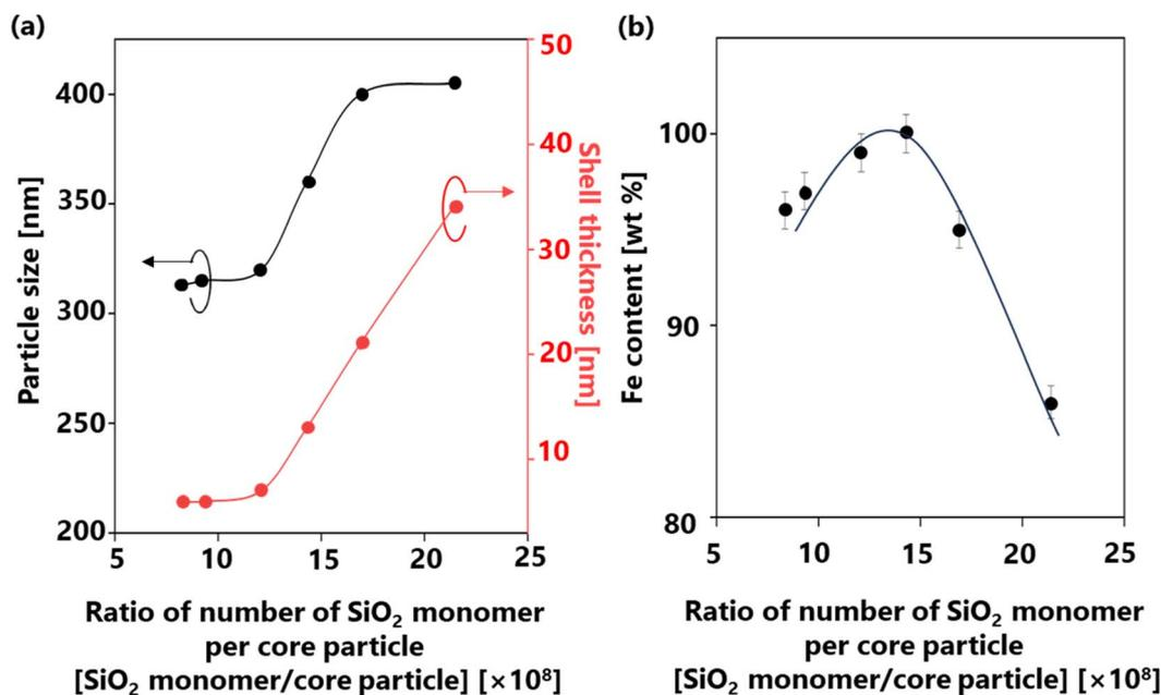
Fig. 7 Correlation between the number of SiO<sub>2</sub> monomer per core particle ratios on the (a) particle size and shell thickness and (b)  $\alpha$ -Fe content in the Fe@SiO<sub>2</sub> particles.
