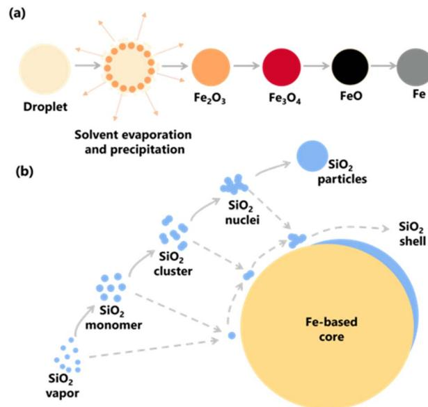
Fig. 1 (a) Schematic representation of the synthesis of Fe particles via spray pyrolysis route and (b) formation of SiO<sub>2</sub> on the surface of the Fe-based core.
