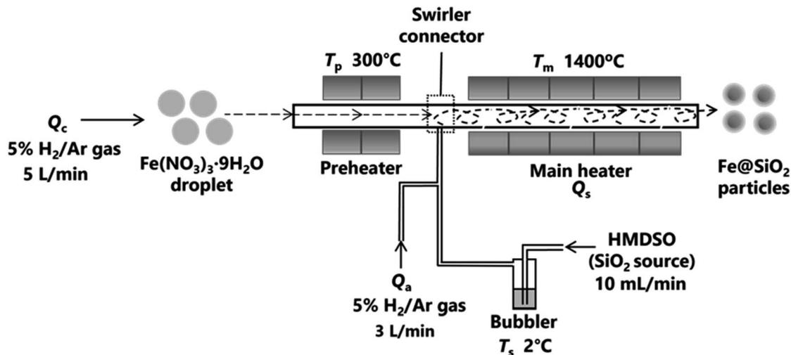
Fig. 2 Experimental setup of synthesizing Fe@SiO<sub>2</sub> particles.
