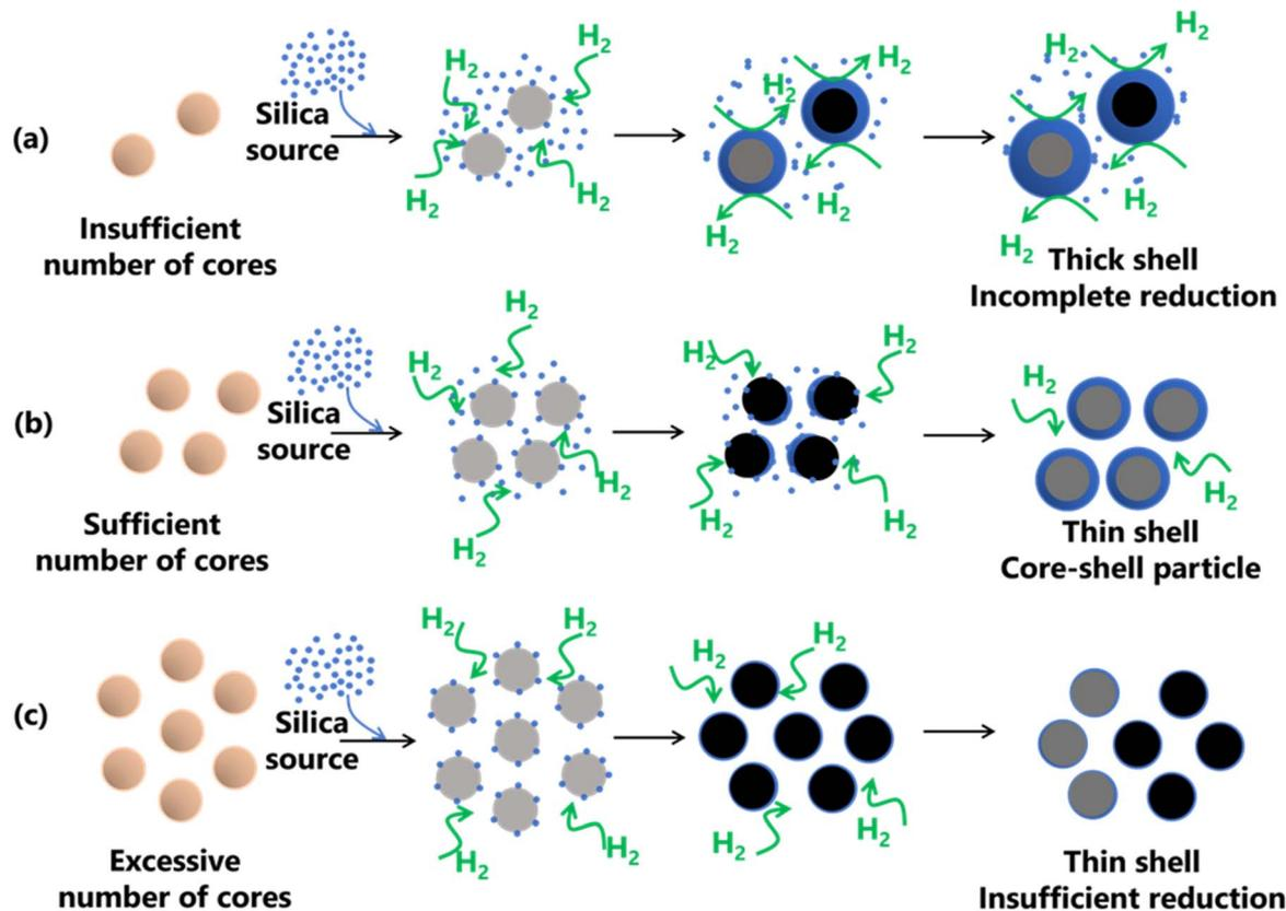
Fig. 8 Proposed mechanism for the formation of SiO<sub>2</sub>-coated Fe with (a) insufficient, (b) sufficient, and (c) excessive number of cores.
