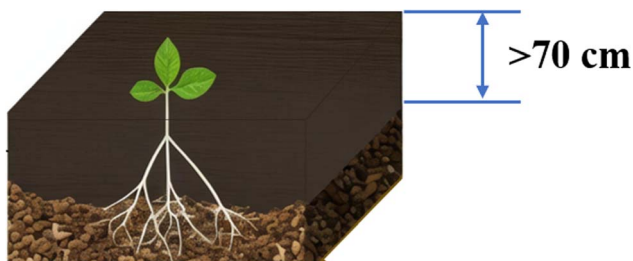
Fig. 3 Schematic diagram of a coal gangue-filled reclamation profile.
