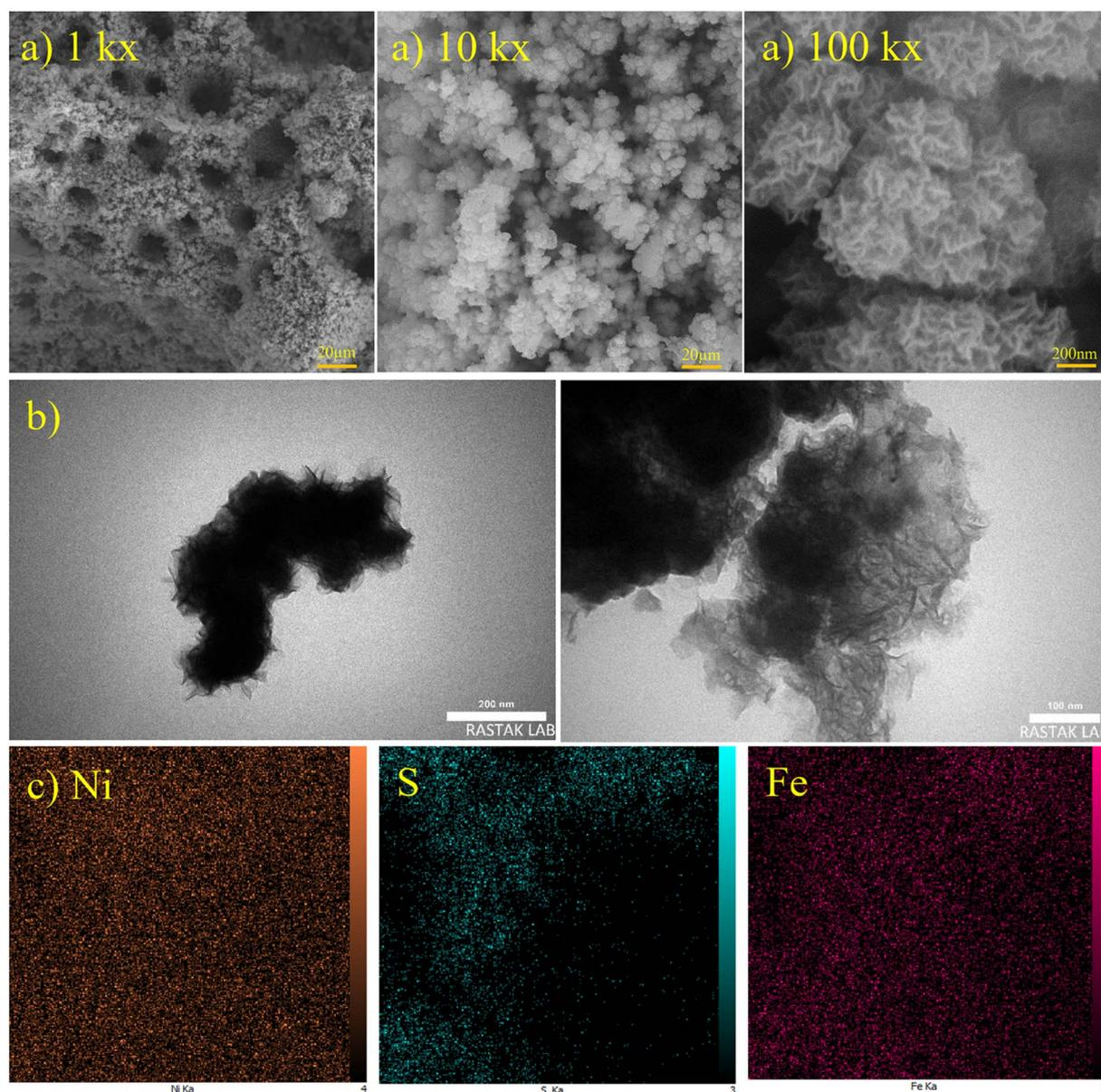
Fig. 5 (a) FESEM images with magnifications of  $1\text{k}\times$ ,  $10\text{k}\times$ , and  $100\text{k}\times$ , (b) TEM images and (c) elemental mapping with magnification of  $5\text{k}\times$  for optimum Ni-Fe-S  $5 \text{ A cm}^{-2}/10 \text{ s}/0.1 \text{ M}$ .
