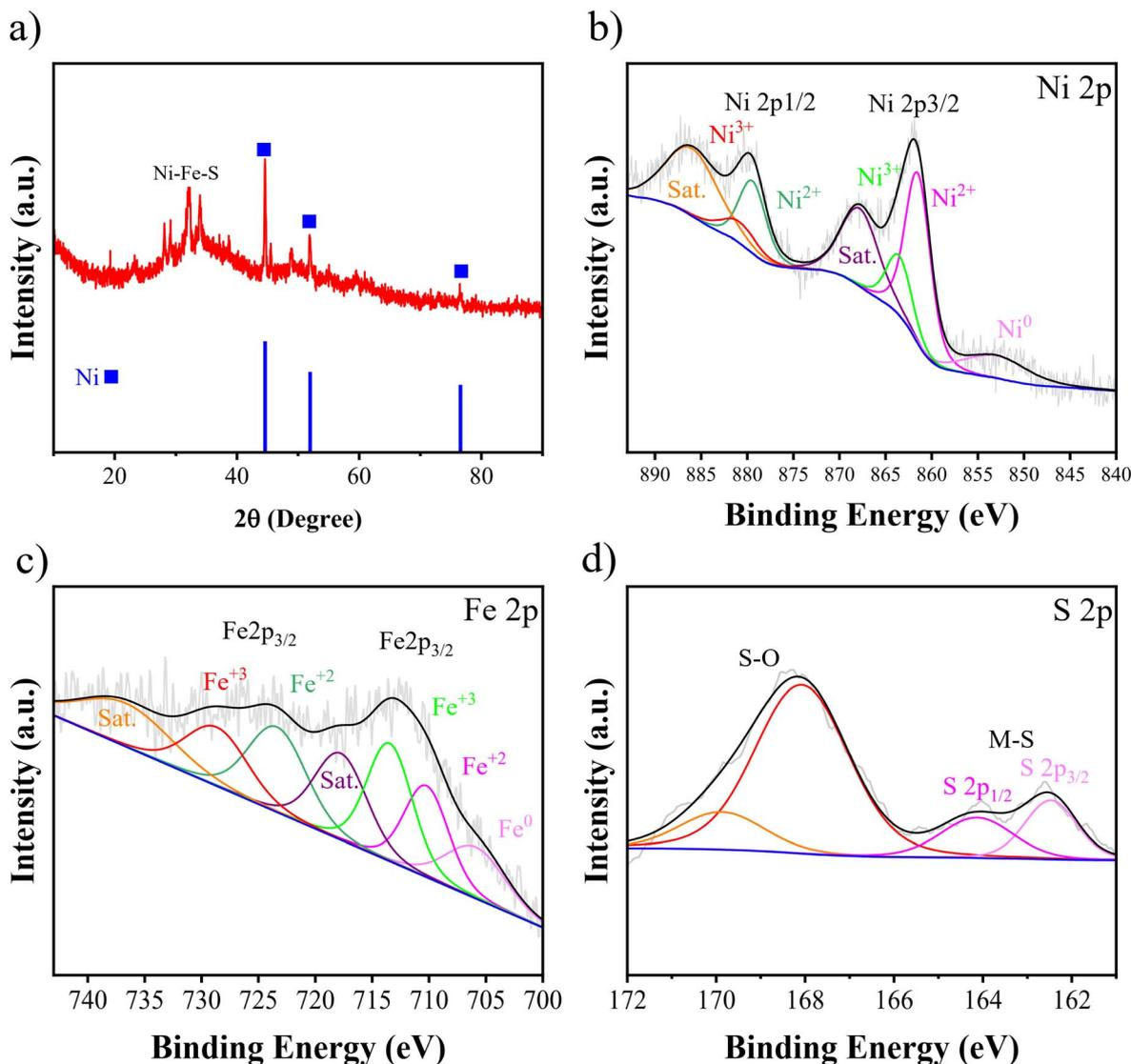
Fig. 6 (a) XRD pattern and high resolution XPS spectra of (b) Ni, (c) Fe, and (d) S for optimum Ni-Fe-S 5 A cm<sup>-2</sup>/10 s/0.1 M.
