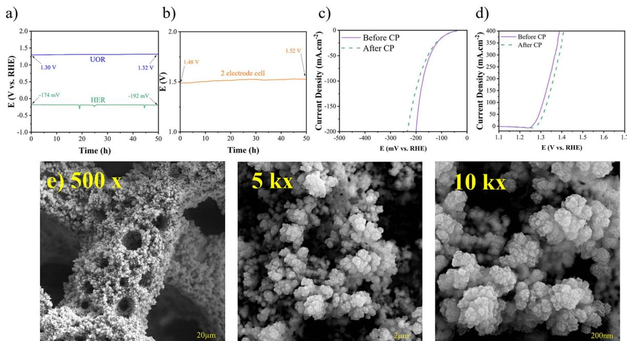
Fig. 12 (a) CP for the HER, UOR, and (b) 2 electrode system recorded at  $100 \text{ mA cm}^{-2}$  for 50 h, LSV curves after CP for (c) HER and (d) UOR, and (e) FESEM images after CP with different magnifications of 500 $\times$ , 1k $\times$ , and 10k $\times$ .
