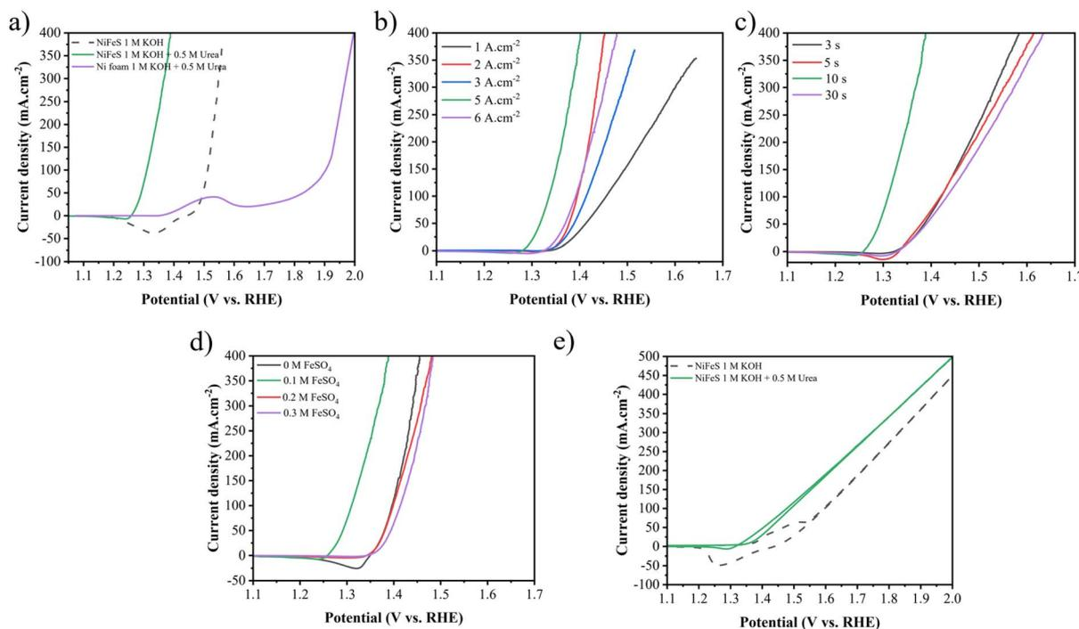
Fig. 8 (a) LSV curves of NF for the UOR and Ni–Fe–S 5 A cm<sup>-2</sup>/10 s/0.1 M for the UOR and OER, LSV curves of the synthesized electrodes with different (b) applied current densities, (c) duration times, and (d) FeSO<sub>4</sub> concentrations in 1 M KOH + 0.5 M urea electrolyte, and (e) LSV curves of 2 electrode system Ni–Fe–S 5 A cm<sup>-2</sup>/10 s/0.1 M||Ni–Fe–S 5 A cm<sup>-2</sup>/10 s/0.1 M towards overall urea oxidation and water splitting.
