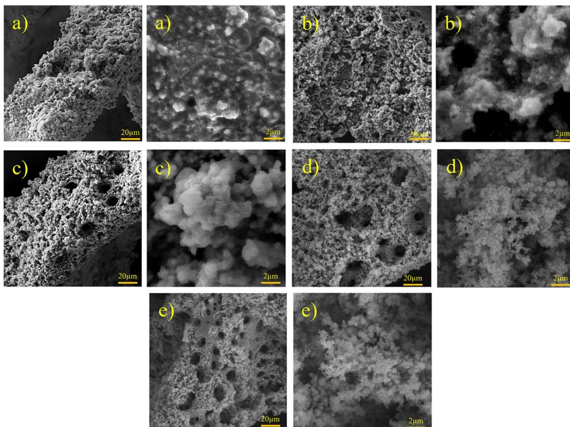
Fig. 2 FESEM images of Ni-Fe-S with magnifications of 1k $\times$  and 10k $\times$  at 10 s, 0.1 M FeSO<sub>4</sub>, and (a) 1, (b) 2, (c) 3, (d) 5, and (e) 6 A cm<sup>-2</sup>.
