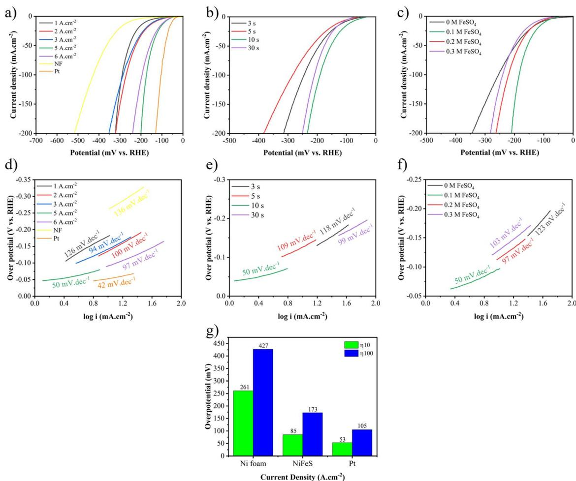
Fig. 7 LSV curves and Tafel curves for the HER at different (a and d) applied current densities, (b and e) duration times, and (c and f) FeSO<sub>4</sub> concentrations, and (g)  $\eta_{10}$  and  $\eta_{100}$  of Pt, NF, and optimum Ni-Fe-S.
