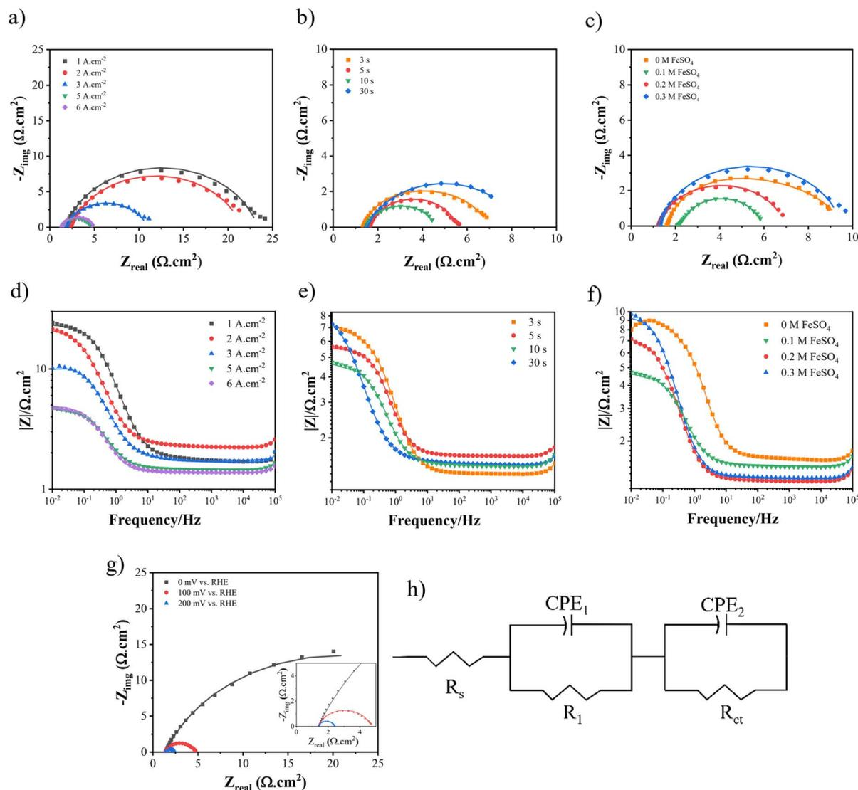
Fig. 10 The Nyquist curves and Bode plots at an overpotential of  $-100$  mV for electrodes fabricated at different (a and d) electrodeposition current densities, (b and e) duration times, and (c and f)  $\text{FeSO}_4$  concentrations, (g) Nyquist curves of Ni-Fe-S  $5 \text{ A cm}^{-2}/10 \text{ s}/0.1 \text{ M}$  at different overpotentials, and (h) equivalent circuit.
