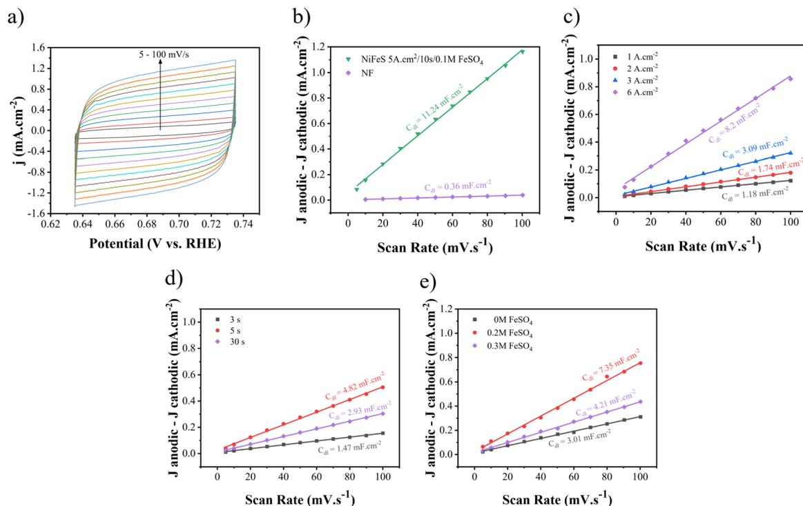
Fig. 9 (a) CV curves with different scan rates (5–100  $\text{mV s}^{-1}$ ) and  $C_{dl}$  plots for (b) optimum Ni–Fe–S and NF and Ni–Fe–S synthesized at (c) different electrodeposition current densities, (d) different duration times, and (e) different concentrations of  $\text{FeSO}_4$ .
