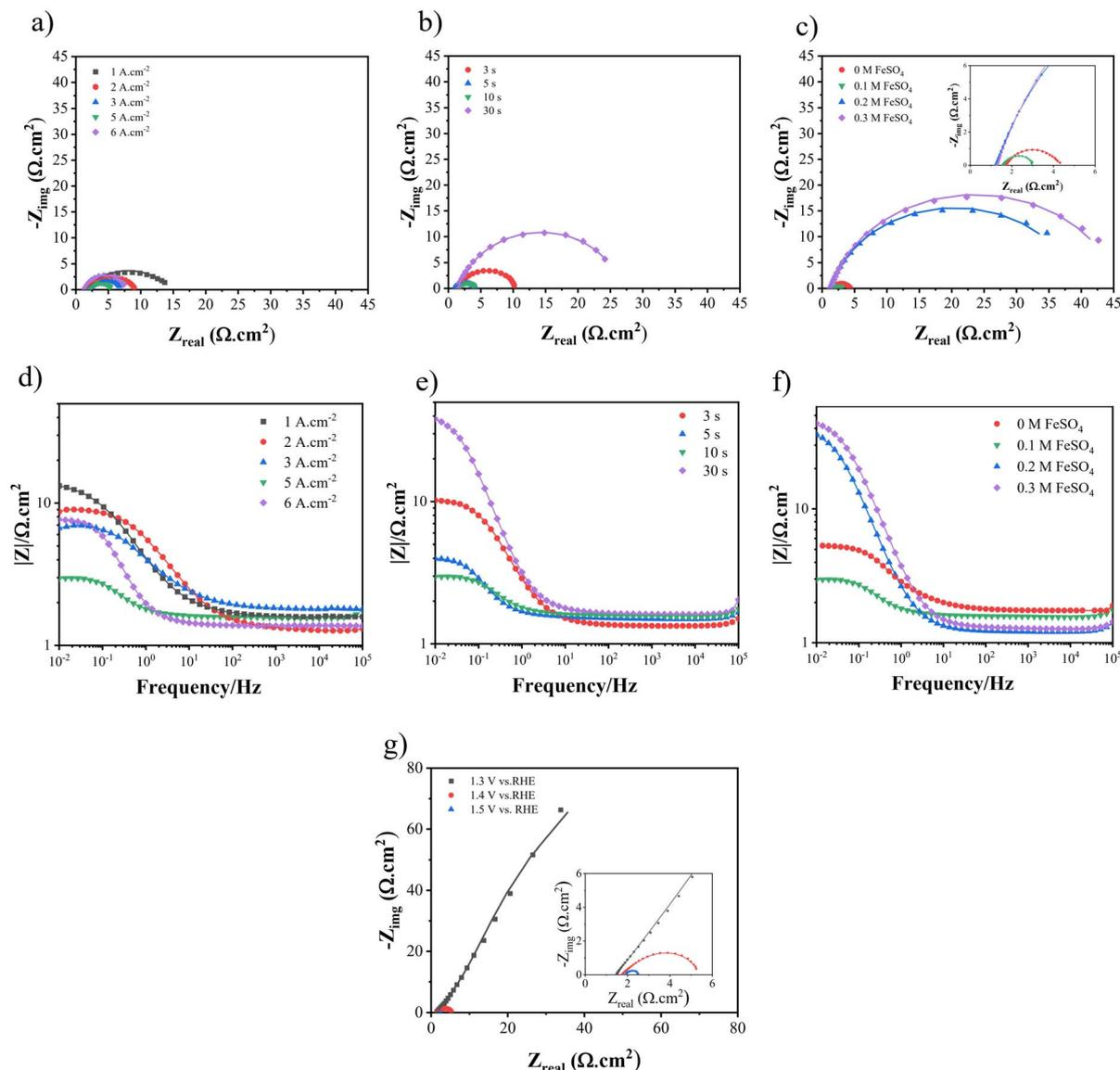
Fig. 11 The Nyquist curves and Bode plots at an overpotential of 1.4 V for electrodes fabricated at different (a and d) electrodeposition current densities, (b and e) duration times, and (c and f)  $\text{FeSO}_4$  concentrations, and (g) Nyquist curves for Ni-Fe-S 5  $\text{A cm}^{-2}/10 \text{ s}/0.1 \text{ M}$  at different overpotentials.
