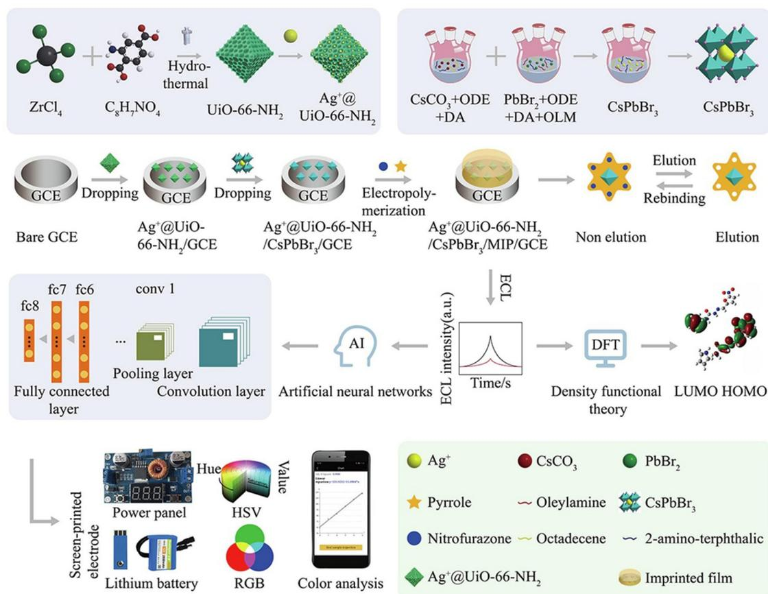
**Fig. 4** A comprehensive illustration of the Ag<sup>+</sup>@UiO-66-NH<sub>2</sub>/CsPbBr<sub>3</sub>/MIP/GCE assembly for a mobile smartphone-based electrochemiluminescence molecularly imprinted polymer (ECL-MIP) system, depicting the intricate steps of preparation, integration of machine learning techniques, and the sensing mechanism. Adapted with permission.<sup>123</sup> Copyright 2022, Elsevier.
