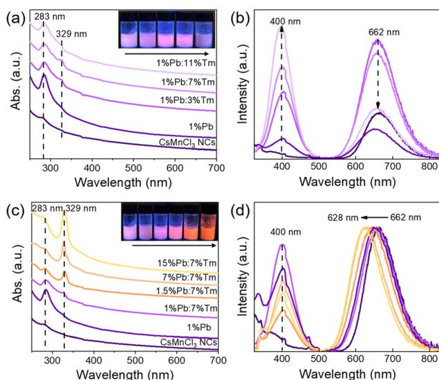
Fig. 5 (a) UV-vis and (b) PL spectra of CsMnCl<sub>3</sub> NCs and Pb/Tm co-doped CsMnCl<sub>3</sub> NCs with changing Tm doping contents. (c) UV-vis and (d) PL spectra of CsMnCl<sub>3</sub> NCs and Pb/Tm co-doped CsMnCl<sub>3</sub> NCs by changing the Pb doping contents. The insets are the luminescence photographs of the above samples under daylight and a 365 nm UV lamp.
