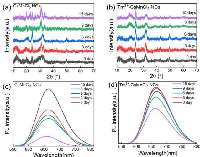
Fig. 6 Time-dependent XRD patterns of (a)  $\text{CsMnCl}_3$  and (b)  $\text{Tm}^{3+}$ - $\text{CsMnCl}_3$  NCs. PL variation of (c)  $\text{CsMnCl}_3$  and (d)  $\text{Tm}^{3+}$ - $\text{CsMnCl}_3$  NCs after different storage times.
