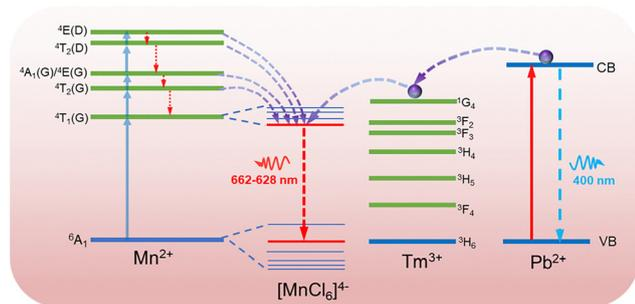
Fig. 4 The schematic diagram for the emission mechanism of undoped and Pb/Tm co-doped CsMnCl<sub>3</sub> NCs.
