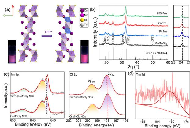
Fig. 1 (a) Schematic diagram of the structure of the undoped and  $\text{Tm}^{3+}$ -doped  $\text{CsMnCl}_3$  NCs. The insets show the comparative photos of red emission under a 365 nm UV lamp. (b) XRD patterns (left panel) and magnified XRD peaks (right panel) of  $\text{CsMnCl}_3$  and  $\text{Tm}^{3+}$ - $\text{CsMnCl}_3$  NCs. The XPS data of (c) Mn 2p and Cl 2p for  $\text{Tm}^{3+}$ - $\text{CsMnCl}_3$  and  $\text{CsMnCl}_3$  NCs, (d) Tm 4d for  $\text{Tm}^{3+}$ - $\text{CsMnCl}_3$  NCs.
