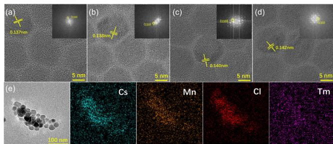
Fig. 2 (a)–(d) HR-TEM images and corresponding FFT pattern of 0%, 3%, 7%, and 13% Tm doping of CsMnCl<sub>3</sub> NCs. (e) TEM and EDS mapping images of Tm<sup>3+</sup>-CsMnCl<sub>3</sub> NCs.
