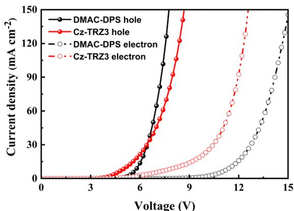
Fig. 5 Hole-only and electron-only devices of DMAC-DPS and Cz-TRZ3. The hole-only device structure is ITO/HAT-CN (5 nm)/TAPC (40 nm)/TCTA (10 nm)/mCBP (5 nm)/DMAC-DPS or Cz-TRZ3 (25 nm)/TAPC (20 nm)/Al (150 nm). The electron-only device structure is ITO/PBPPPhen (20 nm)/DMAC-DPS or Cz-TRZ3 (25 nm)/PPF (10 nm)/PBPPPhen (40 nm)/LiQ (2 nm)/Al (150 nm).
