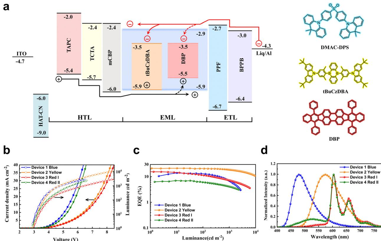
Fig. 1 (a) Energy diagram and molecular structures of emitters adopted in monochrome blue/yellow/red OLEDs. (b) Current density–voltage–luminance ( $J$ – $V$ – $L$ ) curves of monochrome OLEDs. (c) EQE–luminance characteristics of monochrome blue/yellow/red OLEDs. (d) EL spectra of monochrome blue/yellow/red OLEDs at  $100 \text{ cd m}^{-2}$ .
