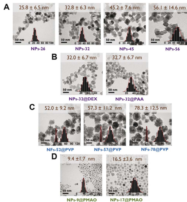
Fig. 1 TEM images and particle size distribution: (group A) uncoated octahedral nanoparticles with sizes between 26 and 56 nm, (group B) 32 nm octahedral nanoparticles with different coatings, (group C) nanoflowers with the same core size (8–10 nm) and coating (polyvinylpyrrolidone) and different particle sizes (52–78 nm), and (group D) spherical nanoparticles with sizes of about 9 and 17 nm coated with PMAO.
