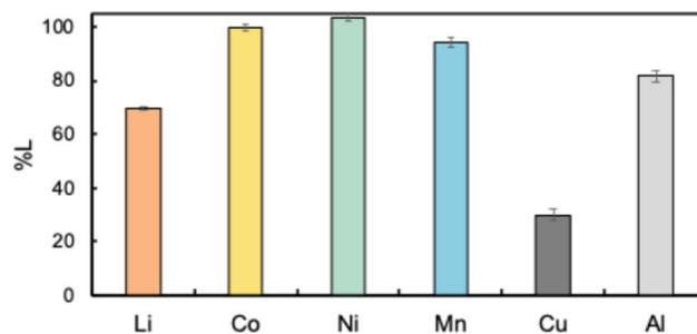
Fig. 6 Leaching efficiencies of the metals from the LiB black mass by 0.6 mol per L D2EHAG in *n*-dodecane with 0.3 mol per L ascorbic acid and a saturated amount of water. Experimental conditions: S/L = 10 g L<sup>-1</sup>, heating at 333 K at 400 rpm for 24 h.
