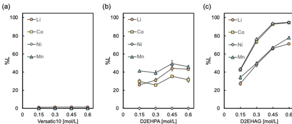
Fig. 3 Leaching efficiencies of the metals from NMC by different concentrations of (a) Versatic10, (b) D2EHPA, and (c) D2EHAG diluted in *n*-dodecane with 0.1 mol per L ascorbic acid and a saturated amount of water. Experimental conditions: S/L = 10 g L<sup>-1</sup>, heating at 333 K at 400 rpm for 24 h.
