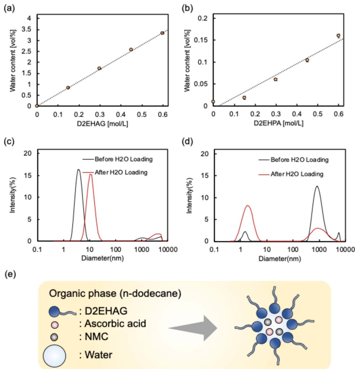
Fig. 4 Saturated water contents in *n*-dodecane containing the extractants (a) D2EHAG and (b) D2EHPA. Particle diameters in *n*-dodecane containing the extractants (c) D2EHAG and (d) D2EHPA. (e) Schematic representation of the expected extractant and water state in the organic solvent.
