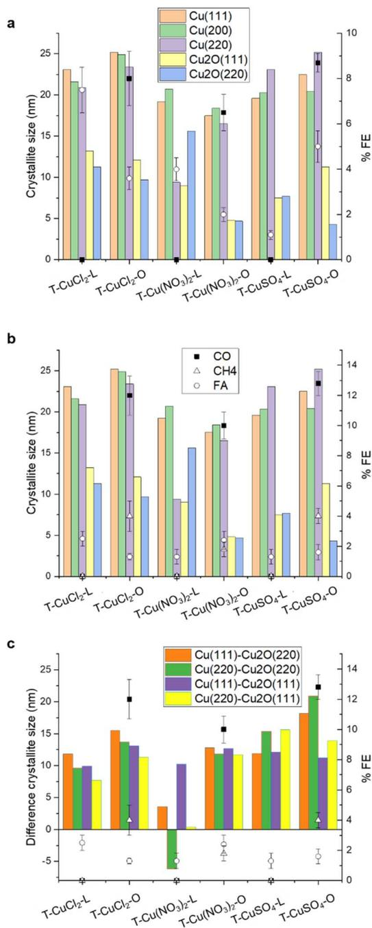
Fig. 7 (a) Correlation between the FE obtained at  $-1.8$  V vs. Ag/AgCl and the size of the planes as indicated, determined by XRD analysis; (b) correlation between the FE obtained at  $-2$  V vs. Ag/AgCl and the size of the planes as indicated, determined by XRD analysis; (c) correlation between the FE obtained at  $-2$  V vs. Ag/AgCl and the difference between the size of the planes as indicated.
