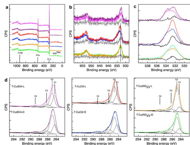
Fig. 4 XPS analysis of the samples investigated using a PHI VersaProbe II (Physical Electronics), equipped with an Al K $\alpha$  (1486.6 eV) X-ray source. (a) Survey spectra; (b) Cu 2p<sub>3/2</sub>; (c) O 1s, and (d) C 1s. The colour code is consistent in this figure as follows: T-CuSO<sub>4</sub>-L (magenta), T-CuSO<sub>4</sub>-O (purple), T-CuCl<sub>2</sub>-L (red), T-CuCl<sub>2</sub>-O (blue), T-Cu(NO<sub>3</sub>)<sub>2</sub>-L (orange), and T-Cu(NO<sub>3</sub>)<sub>2</sub>-O (green).
