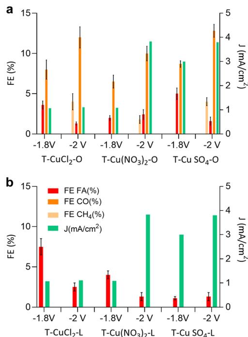
Fig. 6 Current density ( $J$ ), and faradaic efficiency of formic acid (FA), carbon monoxide (CO) and methane ( $\text{CH}_4$ ) of (a) orange peel-derived samples and (b) the lemon peel derived sample after 1 hour of testing at an applied potential of  $-1.8$  and  $-2$  V vs. Ag/AgCl.
