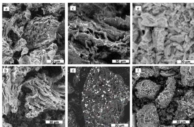
Fig. 1 SEM images recorded with a Phenom ProX Desktop instrument at 10 kV acceleration voltage and at  $\times 2000$  magnification in back-scattered electron (BSE) mode: (a) T-CuSO<sub>4</sub>-O (b) T-CuSO<sub>4</sub>-L (c) T-CuCl<sub>2</sub>-O, (d) T-CuCl<sub>2</sub>-L, (e) T-Cu(NO<sub>3</sub>)<sub>2</sub>-O, and (f) T-Cu(NO<sub>3</sub>)<sub>2</sub>-L.
