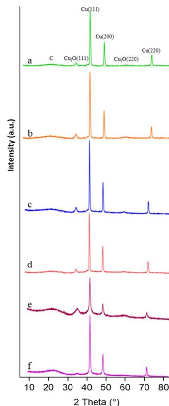
Fig. 2 X-ray diffraction patterns of the as-prepared samples in the  $2\theta$  range of  $10^\circ$  to  $85^\circ$ . From top to bottom: (a) T-CuSO<sub>4</sub>-L, (b) T-CuSO<sub>4</sub>-O, (c) T-CuCl<sub>2</sub>-L, (d) T-CuCl<sub>2</sub>-O (e) T-Cu(NO<sub>3</sub>)<sub>2</sub>-O, and (f) T-Cu(NO<sub>3</sub>)<sub>2</sub>-L.
