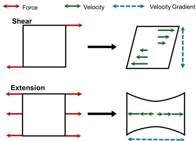
Fig. 3 Illustration of shear and extensional flows.
