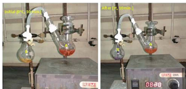
Fig. 3 Mechanistic study (ammonia trapping experiments).
