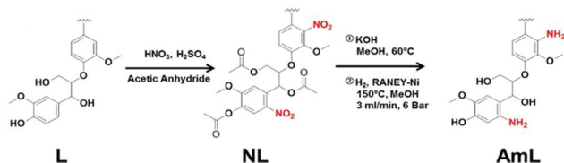
Fig. 2 Synthetic pathway for the conversion of alkali-lignin (L) into amino-lignin (AmL) via aromatic nitration.
