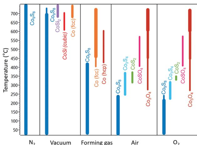
Fig. 6 Summary of crystalline phases observed during *in situ* high-temperature GIXRD measurements performed under different atmospheres. The widths of the lines referring to the different phases represent an estimation on the relative amounts of the different phases based on peak intensities.
