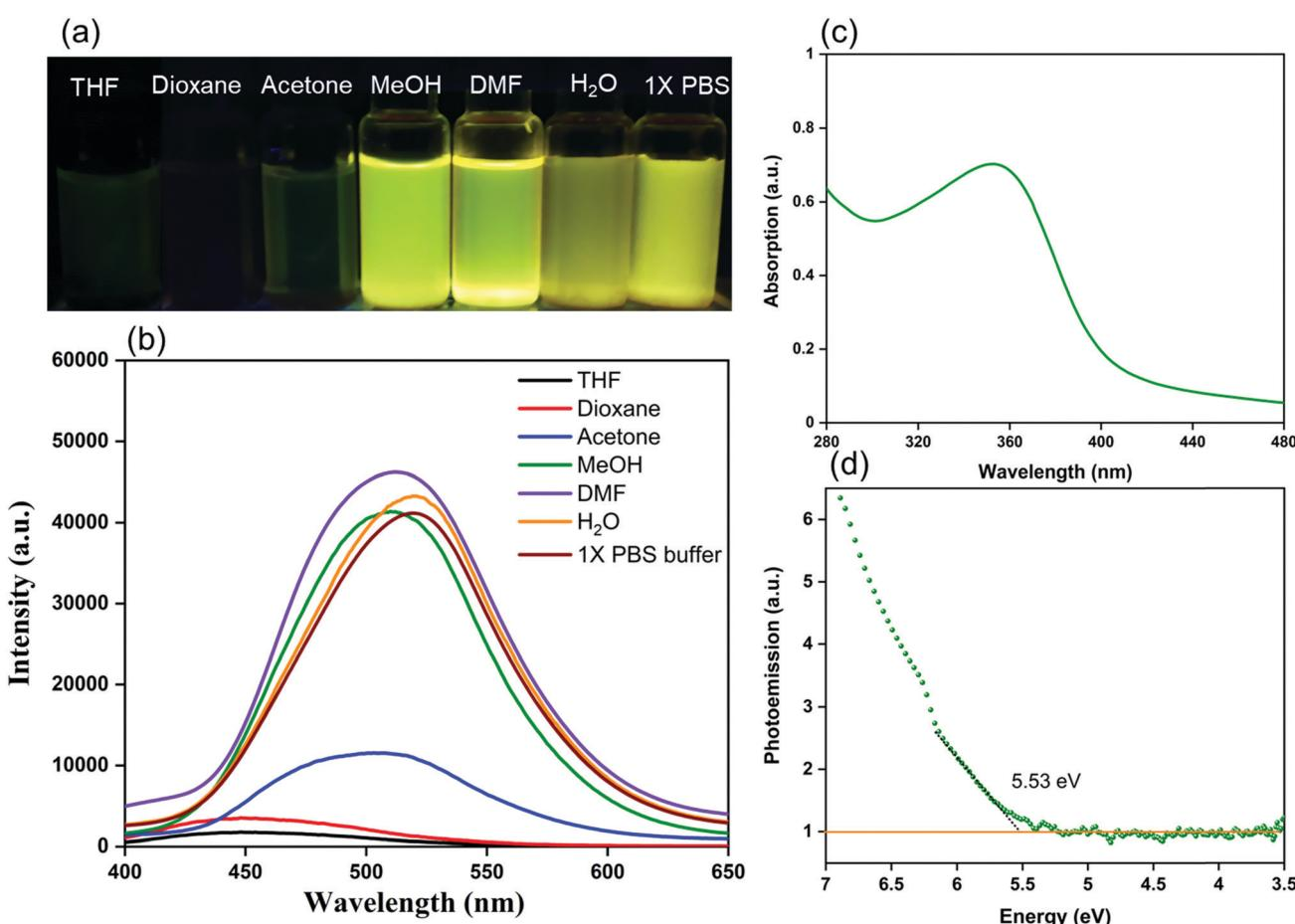
Fig. 4 (a) Photographic images of the **TFPB-DHTH** COF dissolved/dispersed in various solvents upon irradiation with UV light at 360 nm. (b) Fluorescence emission spectra of the **TFPB-DHTH** COF dissolved/dispersed in various solvents (excitation at 365 nm). (c) UV-Vis absorption spectrum of the **TFPB-DHTH** COF dissolved in water (concentration:  $0.125 \text{ mg mL}^{-1}$ ). (d) Photoelectron spectroscopy of the **TFPB-DHTH** COF for calculation of the HOMO energy.
