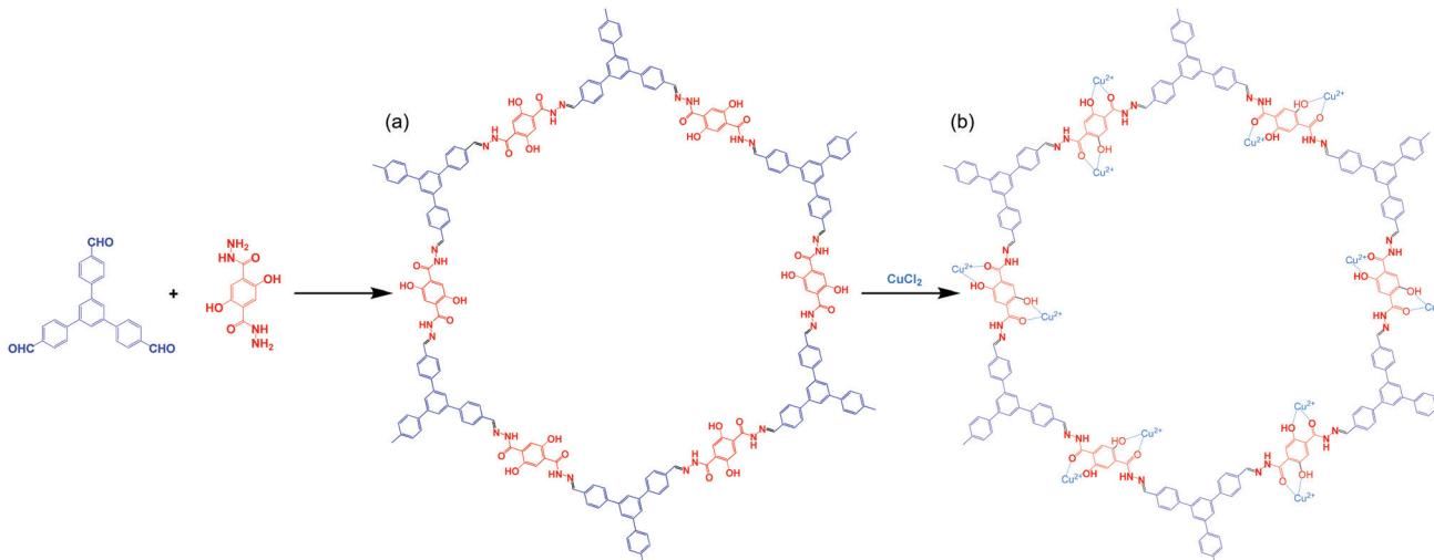
Scheme 1 Synthesis of the **TFPB–DHTH** COF and the **Cu@TFPB–DHTH** COF.
