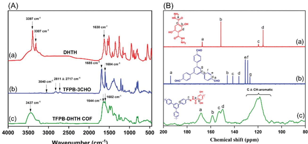
Fig. 1 (A) FTIR spectra of (a) DHTH, (b) TFPB-3CHO, and (c) the TFPB-DHTH COF. (B) <sup>13</sup>C NMR spectra of (a) DHTH and (b) TFPB-3CHO and (c) the solid state <sup>13</sup>C NMR spectrum of the TFPB-DHTH COF.
