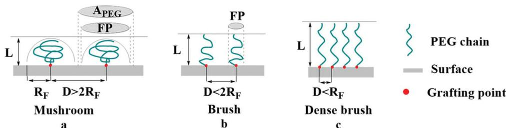
Fig. 4 PEG conformations on a particle surface: (a) Mushroom conformation, (b) brush conformation, and (c) Dense brush conformation. FP: PEG footprint (projected area),  $A_{\text{PEG}}$ : area available to each PEG chain.  $\text{FP} = A_{\text{PEG}}$  in the brush regime, and  $A_{\text{PEG}} > \text{FP}$  in the mushroom regime.
