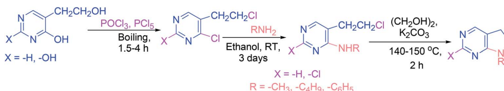
Scheme 19 Synthesis of 5,6-dihydropyrrolo[2,3- d ]pyrimidines.
