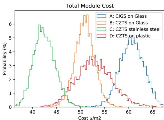
Fig. 2 Total module cost for different product types based on the assumption of 1 GW per year manufacturing volume.
