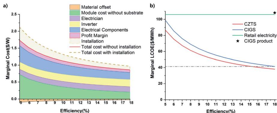
Fig. 5 (a) The marginal breakdown cost of CZTS at different module efficiencies (with and without installation cost); (b) the marginal LCOE of CZTS, CIGS, CIGS commercial products, and retail electricity.
