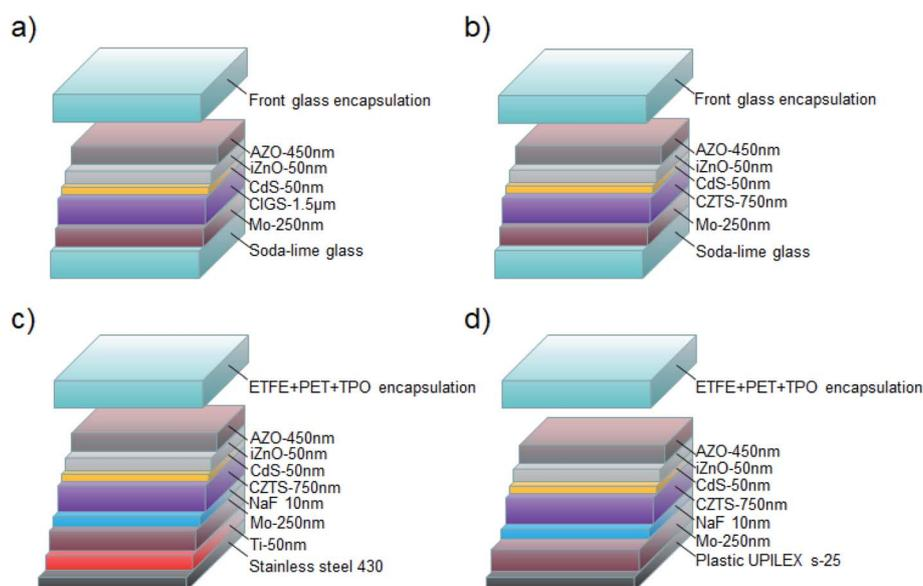
Fig. 1 Structure diagram of process A–D. (a) CIGS on glass, (b) CZTS on glass, (c) flexible CZTS on stainless steel, and (d) flexible CZTS on plastic.
