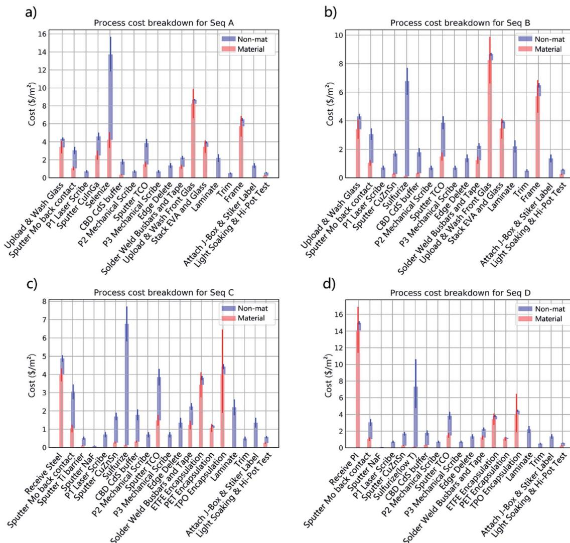
Fig. 3 Cost breakdown with uncertainties for sequences A–D. (a) for CIGS on glass, (b) for CZTS on glass, (c) for CZTS on steel, (d) for CZTS on plastic. The thinner line in each sub-cost presents the upper and lower limits of the cost due to uncertainty.
