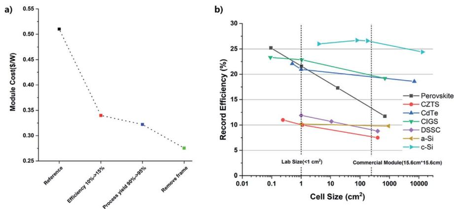
Fig. 4 (a) Strategies for cost reduction in \$ per W; (b) record efficiencies of each technology at different cells per module area.
