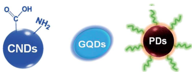
Fig. 2 Illustration of three different types of carbon dots (CDs), from left to right: carbon nanodots (CNDs), graphene quantum dots (GQDs) and polymer dots (PDs).
