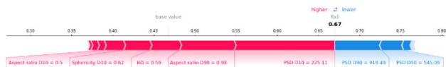
Fig. 16 SHAP force plot of the prediction of the cohesive material from the external validation that was classified as free-flowing by step 1. The red bars of the plot show the drivers that are pushing the classification toward free-flowing and the blue bars show the drivers that are pushing the classification towards non-free flowing.
