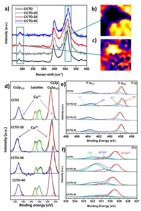
Fig. 4 (a) Raman shifts of the CCTO samples prepared using different PMMA amounts (0, 20, 30, and 40 wt%). (b and c) Raman maps: (b) 510 cm<sup>-1</sup> (CCTO) and (c) 291 cm<sup>-1</sup> (CuO). (d-f) High-resolution XPS spectra of (d) Cu  $2p_{3/2}$ , (e) Ti  $2p_{3/2}$ , and 9f) O 1s for the CCTO samples prepared using different PMMA amounts (0, 20, 30, and 40 wt%).
