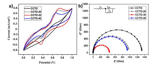
Fig. 6 (a) Cyclic voltammetry curves obtained using CCTO, CCTO-20, CCTO-30 and CCTO-40 as electrodes in 1 M KOH (scan rate =  $25 \text{ mV s}^{-1}$ ). (b) Nyquist plots showing the electrochemical impedance spectroscopy data for CCTO, CCTO-20, CCTO-30 and CCTO-40.
