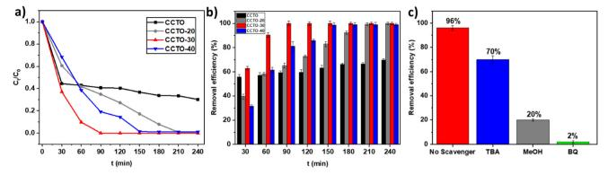
Fig. 7 (a) PCM degradation by electrocatalysis via PMS activation. (b) PCM removal efficiency. (c) Radical scavengers test. TBA: tert-butanol (·OH scavenger); MeOH: methanol (·OH and 'SO scavenger); BQ: p-benzoquinone ('O<sub>2</sub><sup>-</sup> scavenger).
