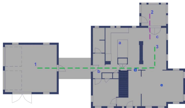
Fig. 2 NZERTF diagram of the first floor. Instruments were located in (1) the garage, (2) the enclosed porch, or (3) the dining room. Locations for (a) cooking, (b) aged smoke injection, (c) chemical cocktail, and (d) fresh smoke. The pesticide was sprayed in (e) the living room. Other chemicals, including ozone ( O_3 ), carbon dioxide ( CO_2 ), and ammonia ( NH_3 ), were injected directly into the supply air flow of the ventilation system (not shown). Dashed lines show sample lines from the garage (green) and porch (purple). Image created by Rileigh Robertson.
